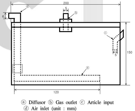
Fig. 1. Schematic diagram of reactor.
