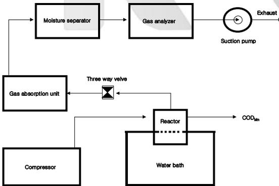
Fig. 2. Schematic diagram of dissolving of organic material.
