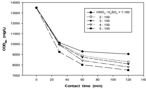
Fig. 4. Organic material dissolving on stripped H<sub>2</sub>SO<sub>4</sub> solution by HNO<sub>3</sub>.
