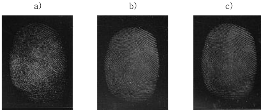
Fig. 2. Color change of nAg and nAg surface modification. a) nAg b) nAg surface modification by DC1501 c) nAg surface modification by DC200.
