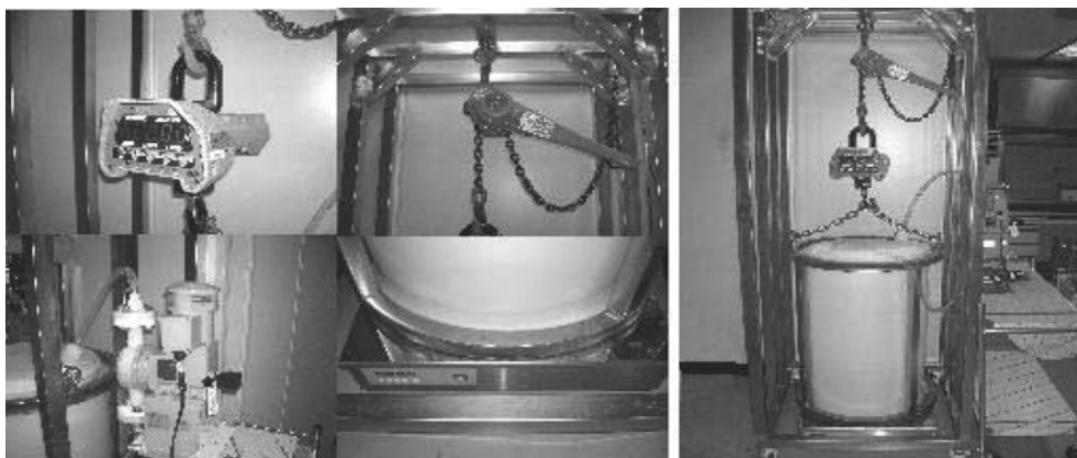
Fig. 1. Apparatus of preparation systems for water-based reference materials.
