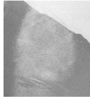
Fig. 7. Latent fingerprint developed on polyester (0 day, Press) by VMD.
