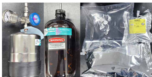
Fig. 1. Gas sample containers used for testing storage stability of the VOCs (from left, Silonite canister, bottle, polymer bags).
