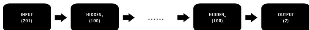
Figure 9. The structure of model in simulation 2. The condition which model has 5 hidden layer is same to the model of simulation 1(see Figure 4). Other models are also same to the model of simulation 1, except the amount of hidden layer.
