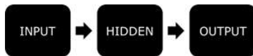
Figure 1. The usual structure of connectionist modeling. The activation is transferred from left to right. The unit sizes of input and output layer are related with the purpose of model, and the computing power of model depend on the unit size of hidden layer.
