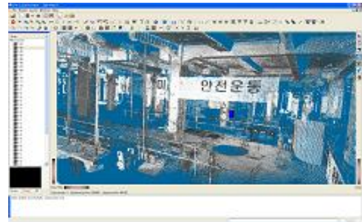
Fig. 6. Scan data acquired at a station of 1 st floor
