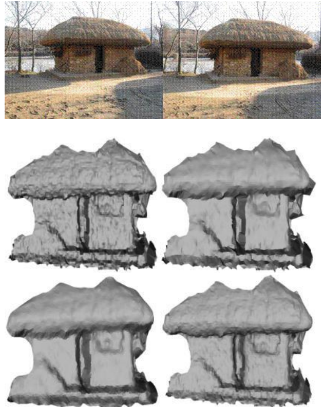
Fig. 13. Reconstructed 3D mesh data from multiple images, (top) Original Image, (top right) 3D reconstructed data, (bottom left) The result using laplacian method[11], (bottom center) the result using median filtering[6], (bottom right) the result by proposed method.
