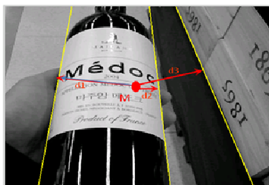
Fig.6. The distance from centre point to each straight line.
