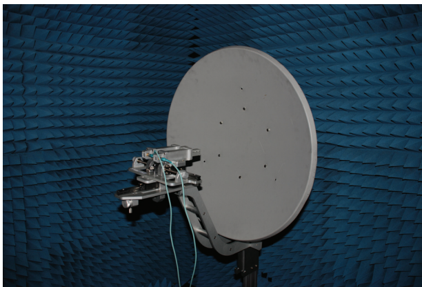
Fig. 2. Antenna under test for near-field antenna measurement
