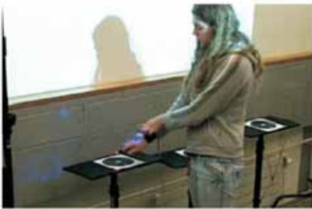
Fig. 4: Registering an object using touching. A user is locating a gesture input device (mWire) at the location of the object and registering the positional data to the system by pressing the button of the device.
