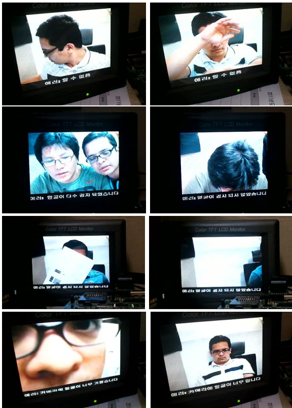
Fig. 8. Some captured images while testing the system for image verification, message at the bottom indicates error frame
