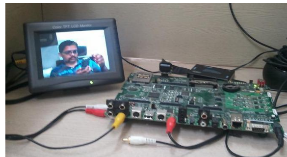
Fig. 1. DaVinci processor board with color LCD monitor
