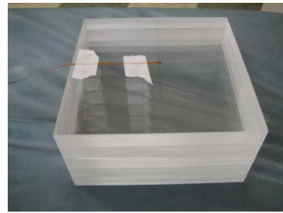
Fig. 1. Insertion of the MOSFET detector in the PMMA phantom
