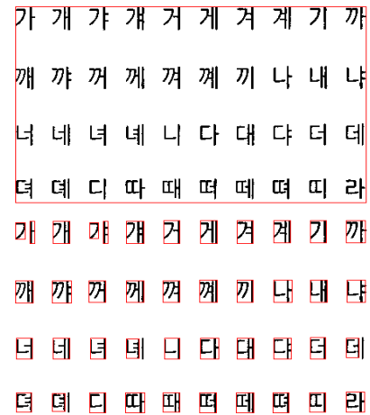
Fig. 15. A sample result of the proposed character labeling method, the first line is the segmented characters, the second line is the recognized character using the OCR system trained by synthetic data and the third line is the labeling result after applying substring matching method. In the third line, the black characters are correctly recognized by the OCR system, and the red characters are revised using Levenshtein distance as presented in step 3 of the substring matching method.
