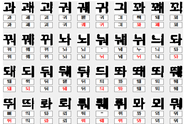
Fig. 15. A sample result of the proposed character labeling method, the first line is the segmented characters, the second line is the recognized character using the OCR system trained by synthetic data and the third line is the labeling result after applying substring matching method. In the third line, the black characters are correctly recognized by the OCR system, and the red characters are revised using Levenshtein distance as presented in step 3 of the substring matching method.
