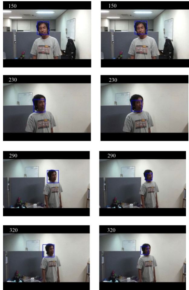
Fig. 8. Comparison without scaling and with scaling in left and right column respectively with same frame number. The rectangle shows the face position.
