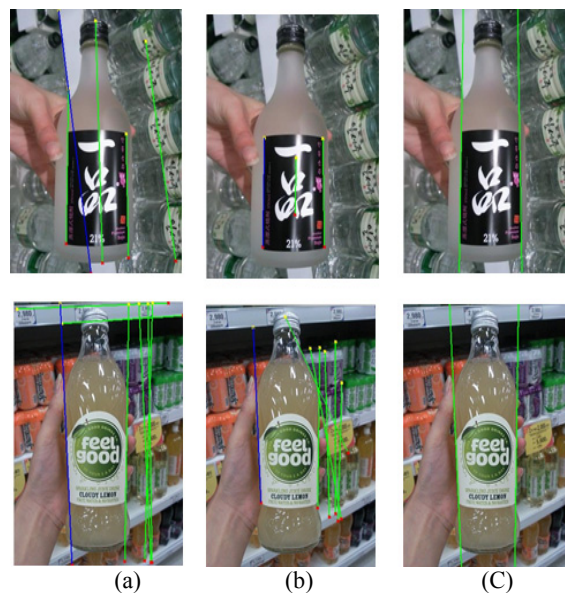
Fig. 9. Comparison of the results of the line detection (a) without and (b) with applying the saliency map, respectively and (c) the final straight line detection results after selecting two similar lines
