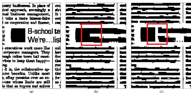
Fig. 4. (a) Binary Image, (b) Smoothing by ARLSA, (c) Smoothing by proposed ARLSA
