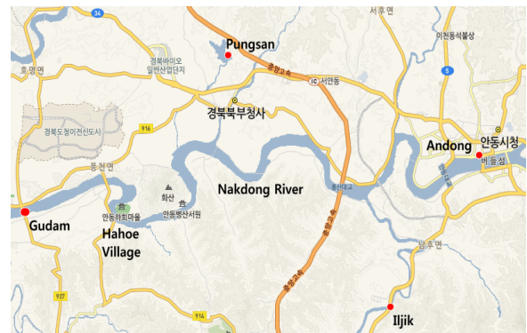
Fig. 2. The map of Andong region. Red circles indicate the locations of water level gauge at "Gudam" and rainfall gauges at "Pungsan", "Iljik", and "Andong"
