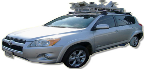
Fig. 1. Measurement devices for inspection of road condition on the express way (MMS)
