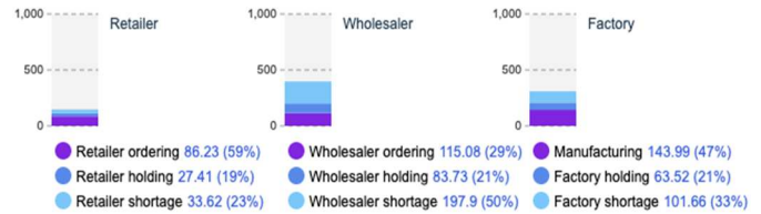
Figure 1: Mean Daily Cost of the Supply Chain (Sourced from the Author's Analysis in Anylogic)
