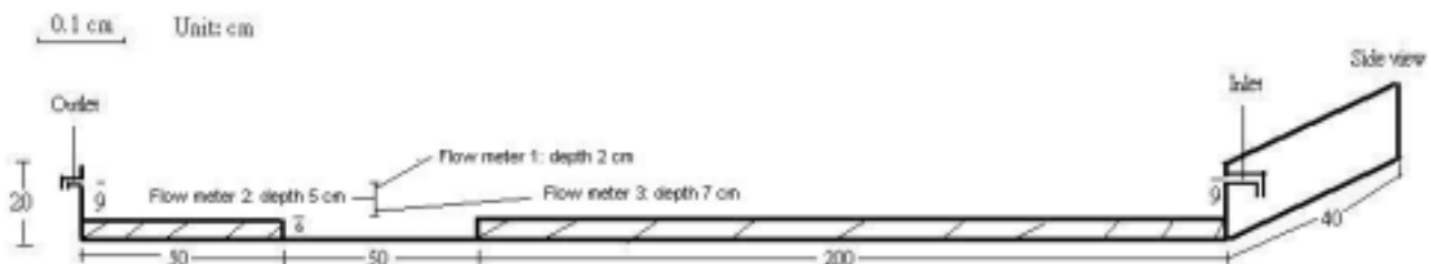
Fig. 1. The setup of the flume apparatus. Note that the depth of the flow meter position is denoted from the water surface.
