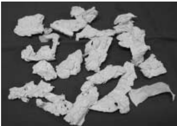
Fig. 2. Deep freeze-dried cellulose membrane after purification.
