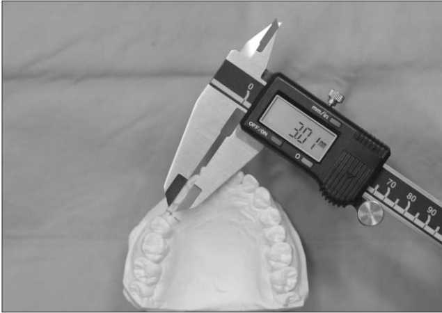
Fig. 3. Measurement of ridge dimension. Immediate postoperation and 4-6 months after operation study models were measured to evaluate the ridge dimensional change using digital caliper
