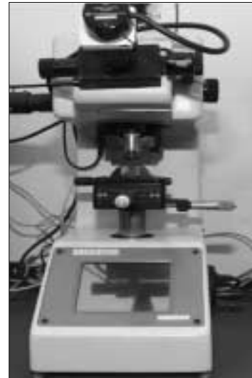
Fig. 4. Knoop hardness tester (MMT-7, Matsuzawa, Japan).
