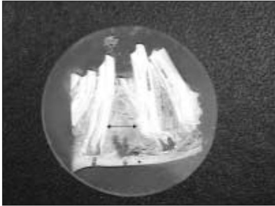
Fig. 3. Sample surface of burnished mandibular body for micro-hardness test.
