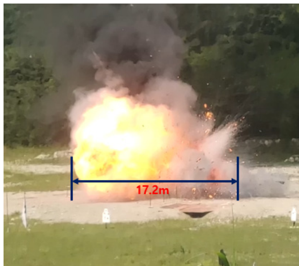
Fig. 6. Fireball ( p_{H_2} = 70 MPa, V = 52.2 L, m_{H_2} = 2, 11 kg)
