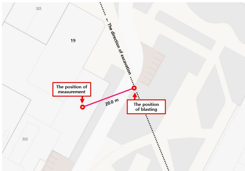
Fig. 3. The location of blasting vibration measurement
