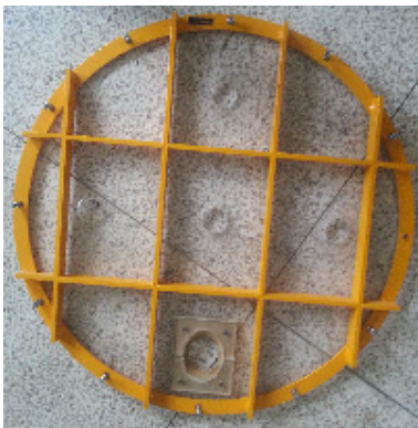
Fig. 6. Prevention frame of bulging
