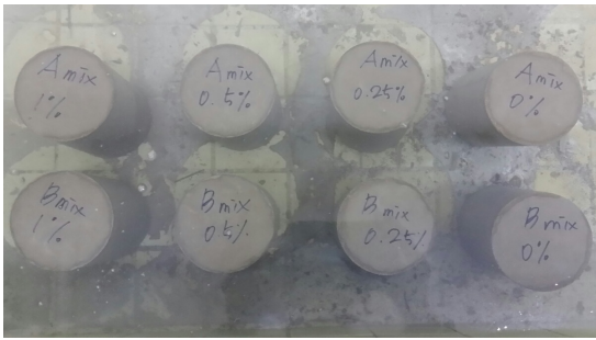
Fig. 2. Immersion of specimens for moisture absorption test
