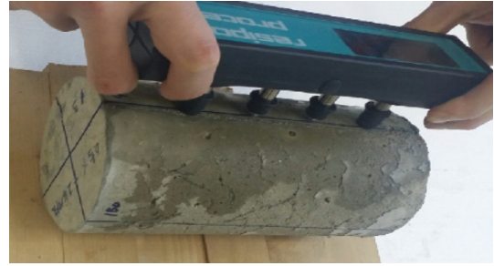
Fig. 4. Surface resistivity measurement
