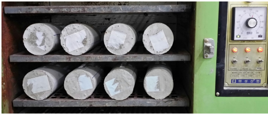
Fig. 1. Drying specimens for moisture absorption test
