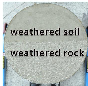
Fig. 7. Mixed ground of weathered soil and rock
