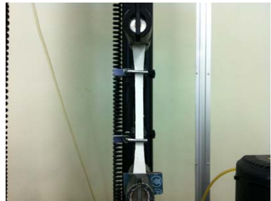
Fig. 3. Tension test for TSL (Chang et al., 2015)
