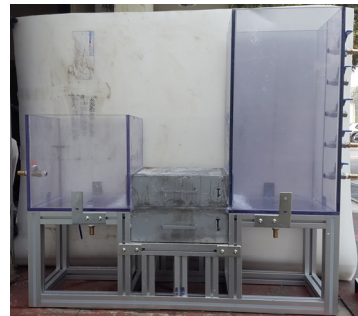
Fig. 3. A typical flow rate testing equipment including shotcrete & concrete lining specimens
