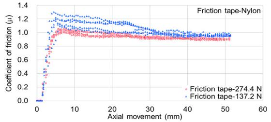
Fig. 8. Friction tape-Nylon friction test [N=137.2, 274.4 N]
