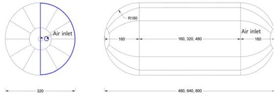
Fig. 12. Inflater general dimensions (1.5D, 2D, 2.5D)
