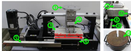
(1) Weight holder for implementation of normal force, (2) Load cell, (3) Sliding specimen, (4) Sliding plate, (5) LVDT, (6) Plate lip, (7) Fabric holding fixture, (8) Load cell, (9) Linear actuator for implementation of horizontal force, (10) Normal weight
