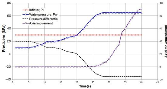
Fig. 13. Model tunnel friction test results
