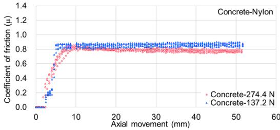
Fig. 6. Concrete-Nylon friction test [N=137.2, 274.4 N]
