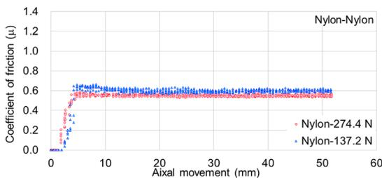
Fig. 7. Nylon-Nylon friction test [N=137.2, 274.4 N]
