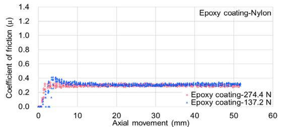
Fig. 9. Epoxy coating-Nylon friction test [N=137.2, 274.4 N]
