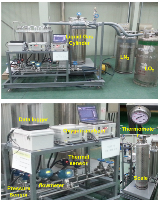
Fig. 2. Equipment for liquid air mixture experiment
