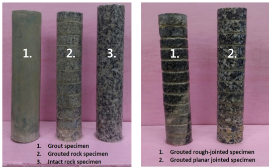
(a) Grout curing experiment (b) Joint roughness experiment
