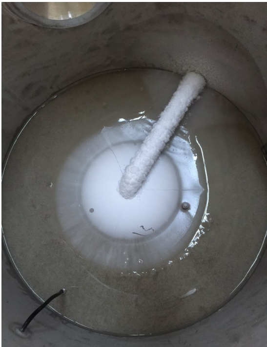
Fig. 8. Frozen surface of soil sample after freezing chamber test
