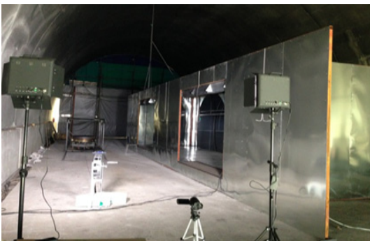
Fig. 4. View of a full-scale fire test (before test)
