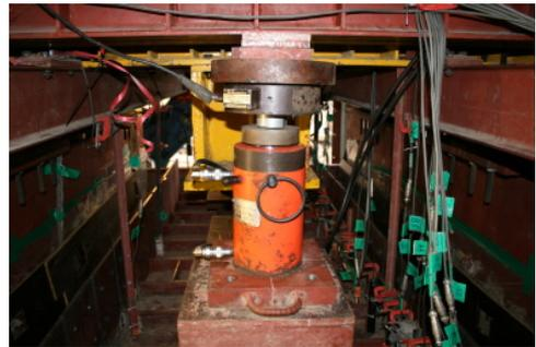
(b) Loading on the plate with hydraulic cylinders
