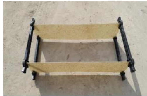
(b) Assembly of GFRP plate
