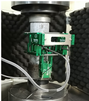
(a) Rock specimen with axial and lateral strain device
