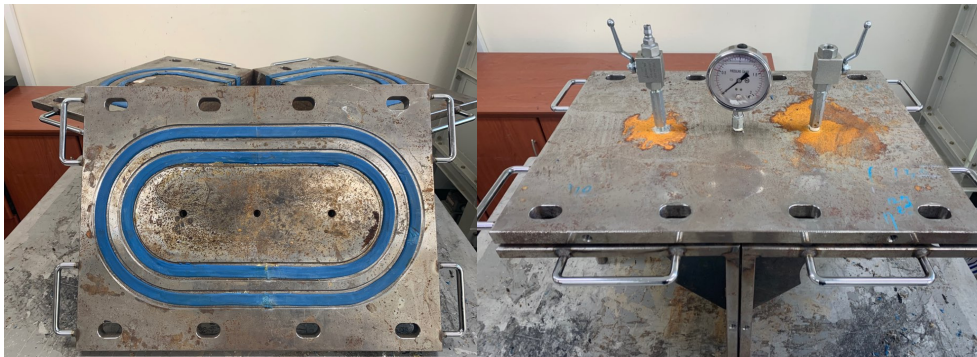
Fig. 3. Test apparatus for hydrophilic rubber waterstop (2 layer)
