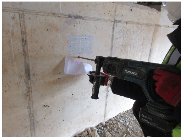
Fig. 1. Overview of carbonation depth test
