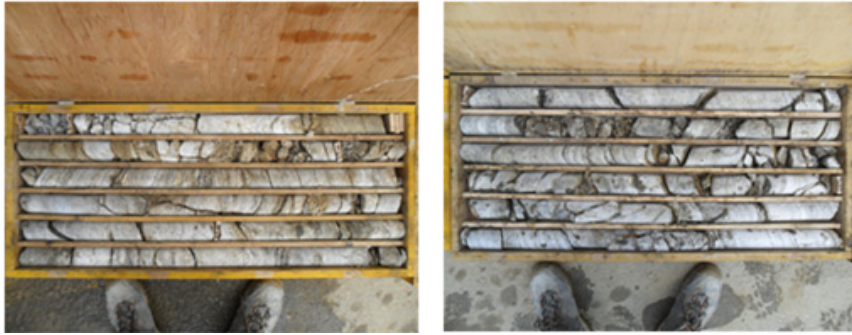
Fig. 9. Core extracted from the borehole
