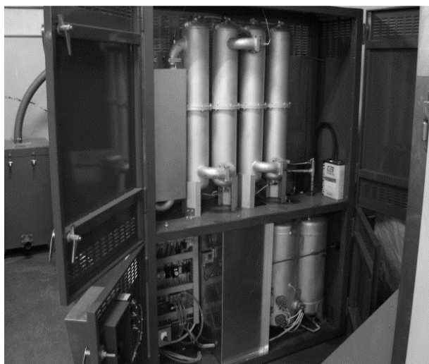
Figure 2: The View of VOCs Control System with Combustion Catalytic Oxidation
