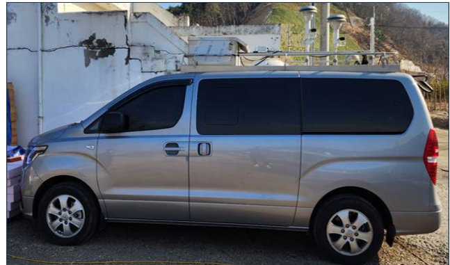
Figure 5: Mobile Air Quality Measurement System Outdoor Area
