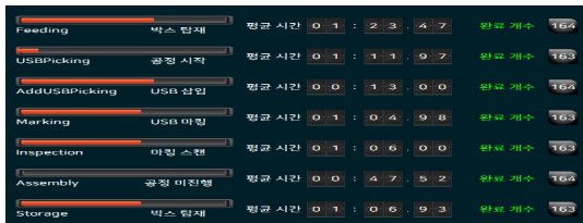
[Fig. 8] Display of process progress
