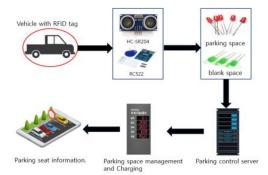
Figure 2 : Intelligence Parking Lot Control System Diagram
