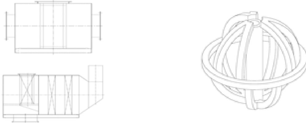
Figure 6: Gas-liquid Separation Device and Filler
