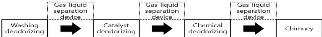
Figure 2: Chemical liquid deodorizer air flow by liquid catalyst
